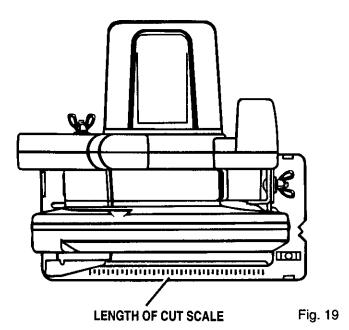
A length of cut scale has been provided on the base of your saw. It is parallel with the saw blade and can be used to measure the distance into material the blade has cut. **Note:** Six inches is the maximum length of cut that can be measured. Also, it is accurate only when the depth of cut is set at full maximum depth,
